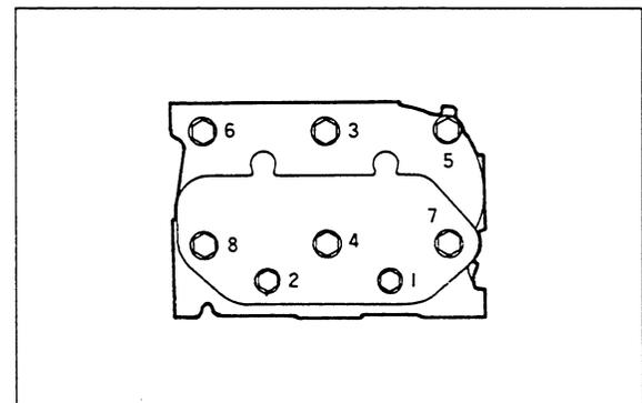
Sequence for Tightening Cylinder Head Bolts
