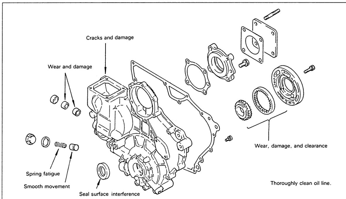
Inspection of Gear Case and Oil Pump
