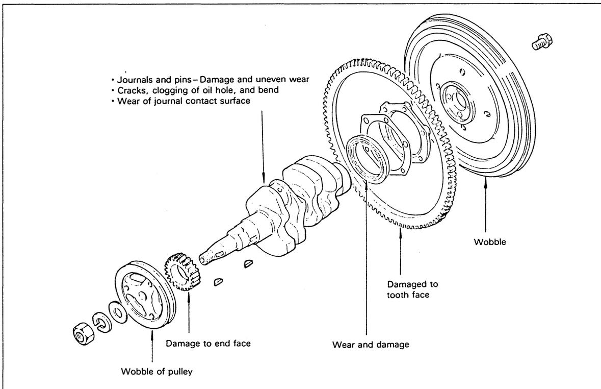
Inspection of Crankshaft and Flywheel
