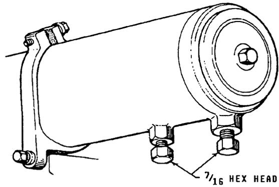
Heat Exchanger Drains
