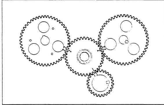
Timing Gears in Alignment with Each Other
