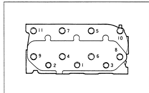
Sequence for Tightening Cylinder Head Bolts
