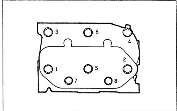
Sequence for Loosening Cylinder Head Bolts
