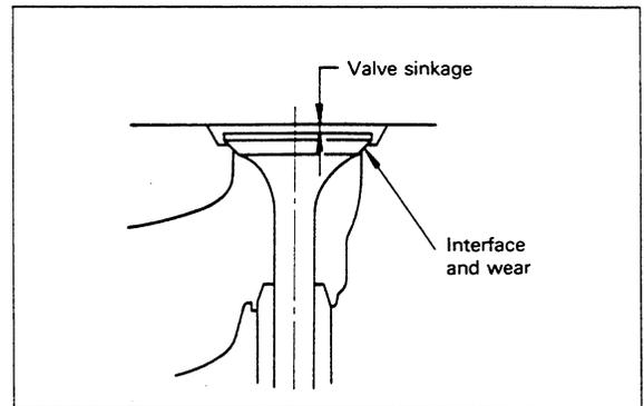
Checking Valve Sinkage
